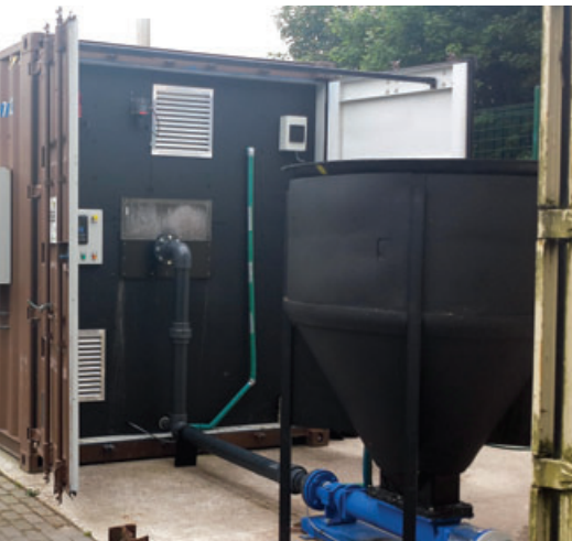
The Lancaster Microbrewery is anaerobically digesting its spent grain and hops from the brewing process.
